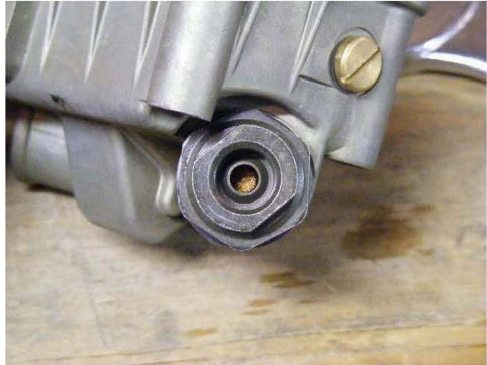
Begin by carefully removing the fuel inlet fitting using the appropriately sized open-end wrench. Most Holley carburetors (and many Quadrajets as well) will require a 1" wrench. Be sure to use a quality wrench to avoid damaging the fitting.
