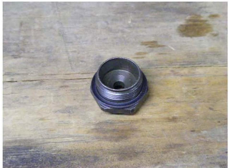
Next, place the small filter gasket into the fitting, making sure it sits flush into the cavity. I have the gasket propped up in the fitting here just to make it easier to see.
