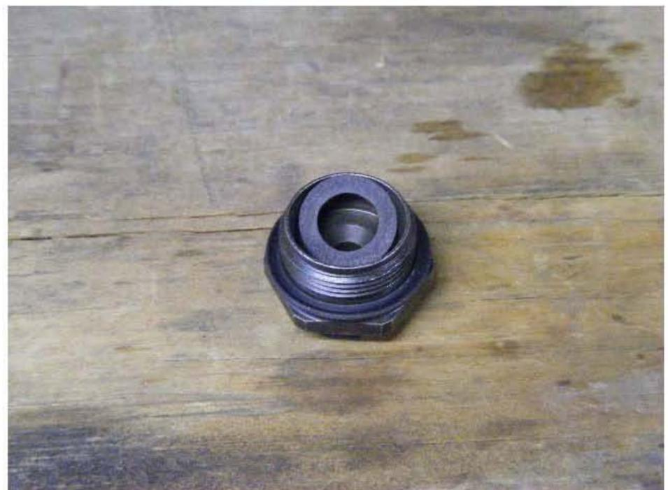
**Next you will install the filter element, making sure to install it in the correct direction as seen here.**
