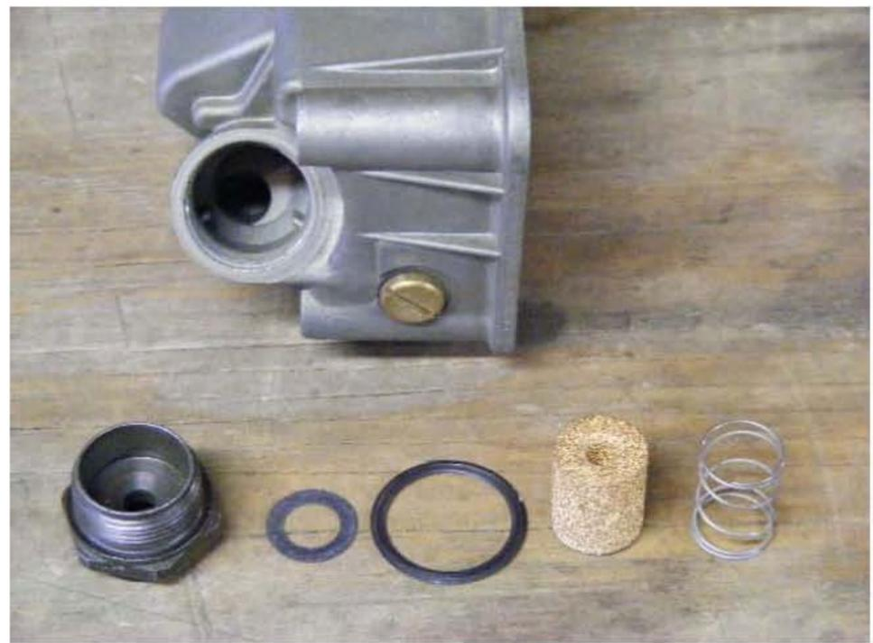
Once you have removed the old filter, clean the inlet fitting as required and begin the reassembly process by placing the large gasket over the threads on the inlet fitting as seen here.
