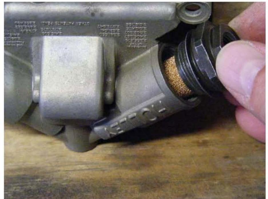
**And there you have it, that's all there is to replacing a fuel filter. Again, I personally recommend that fuel filters should be replaced once a year regardless of how often the vehicle is in use. Condensation and certain additives can quickly foul a filter, so they should be considered a routine maintenance item. Besides, they're cheap insurance compared to the cost of a full rebuild if a carb gets fouled by dirty fuel and debris.**
