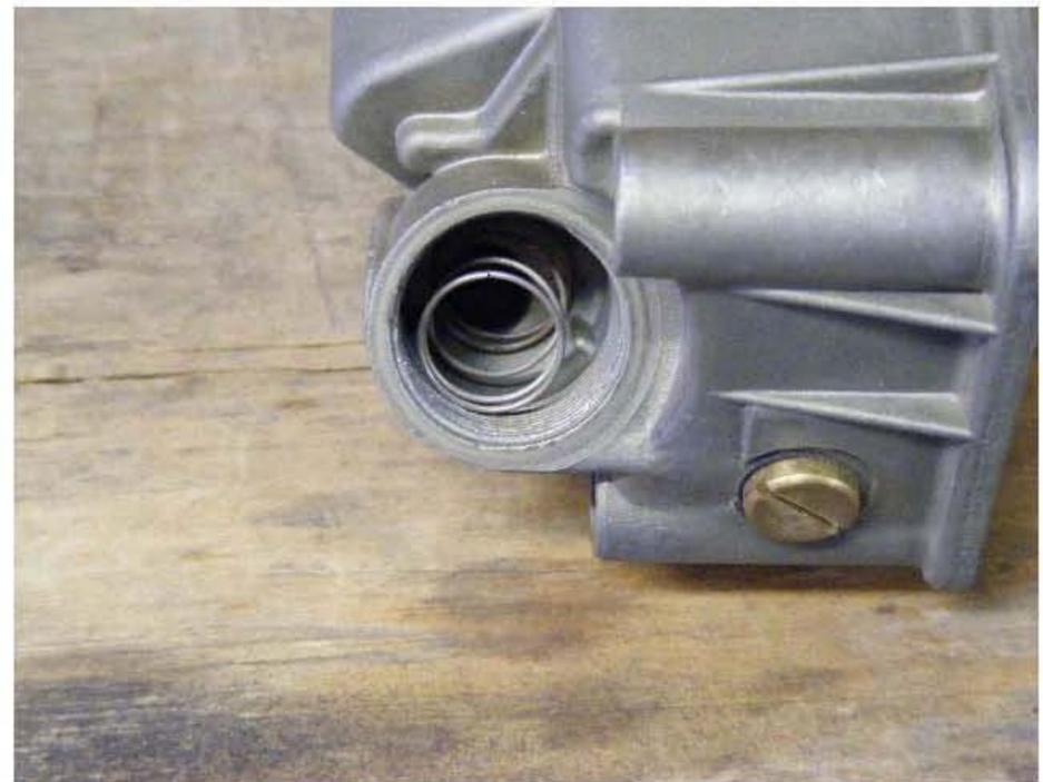
**The final step is to carefully reinstall the filter and inlet fitting assembly. A drop of oil on the inlet fitting threads is a good idea, and you must make certain the bypass spring does not get turned sideways in the cavity as you compress it to start the threads. ALWAYS start the fitting by hand for 2-3 turns, then you can use a wrench to fully tighten the fitting.**
